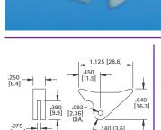
complete with stainless steel spring pin.
